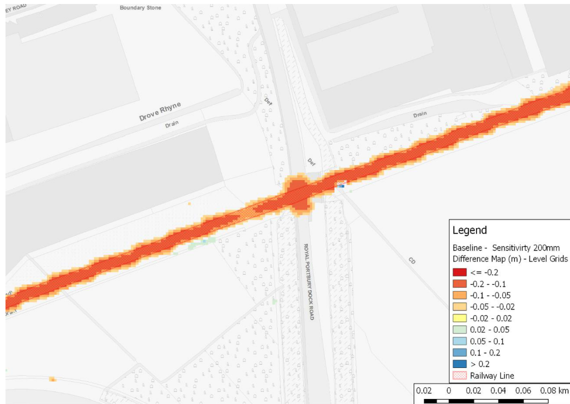
Figure 16: Flood level difference map for comparison between the Baseline run and the 200mm railway level sensitivity run at Royal Portbury Dock Road (1% AEP in 2115).
